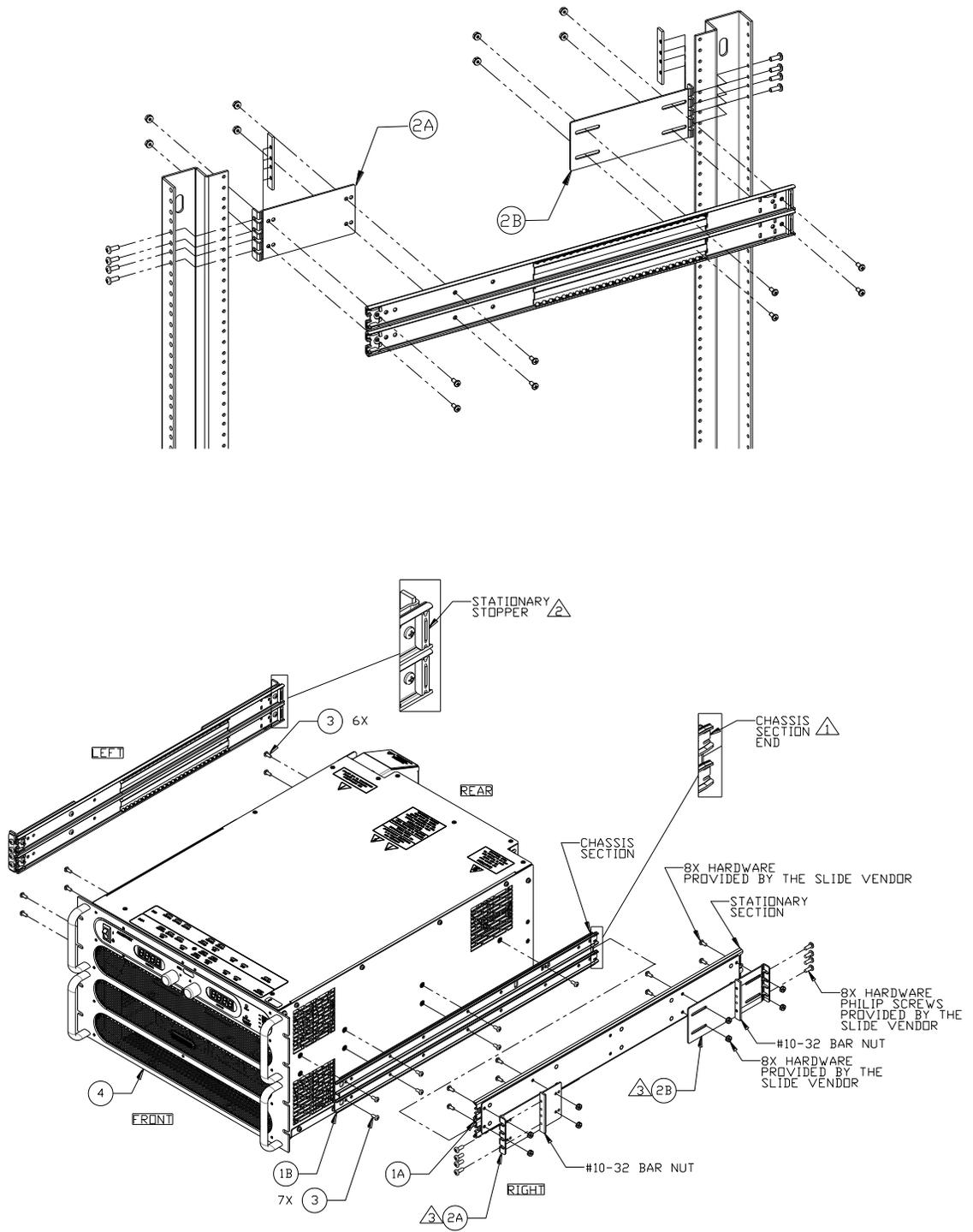
**Figure 2-2. Rack Mount Assembly for 6U Models**
