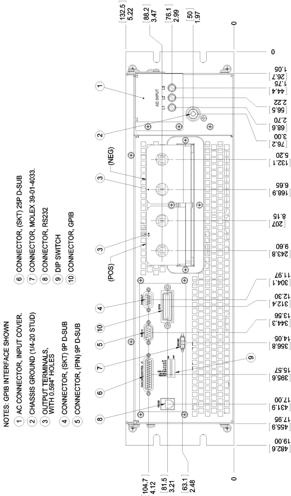
Figure 2-9. Rear Panel, GPIB Option, 3U Models 10V-30V
