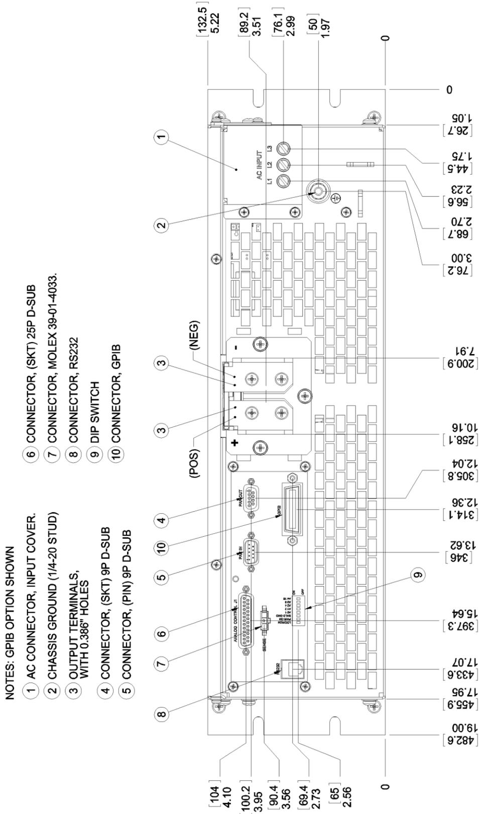
Figure 2-12. Rear Panel, GPIB Option, 3U Models 40V-600V
