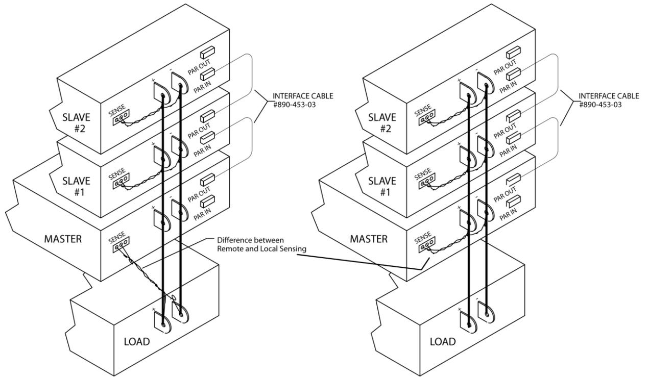
PARALLEL WITH REMOTE SENSING (block diagram)
