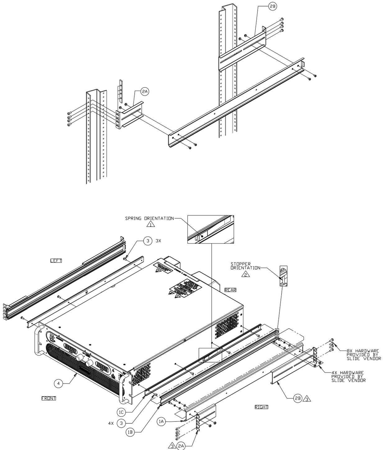
Figure 2-1. Rack Mount Assembly for 3U Models
