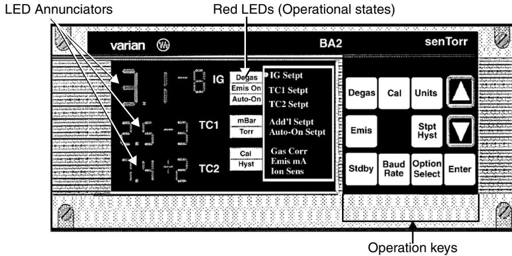
Figure 1-1 senTorr Gauge Controller Front Panel
