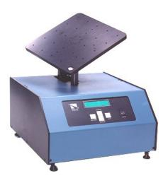
switch, LCD display, and four keys: run/menu, increase, decrease, and enter. Full computer controlled automation can be accomplished with an RS-232 (standard) or IEEE-488 (optional) interface.
