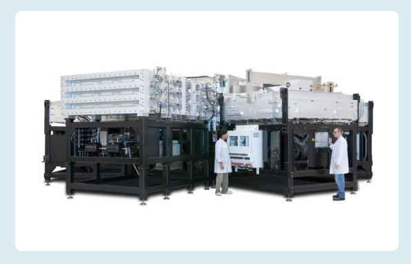
**PECVD a-Si** systems from AKT have been first to market for each generation from Gen 2 to Gen 10 for the TFT-LCD industry. AKT's proven architecture and processes optimize yield, productivity, and reliability; making us the market leader in Flat Panel Display PECVD equipment with over 750 PECVD systems in the field.
