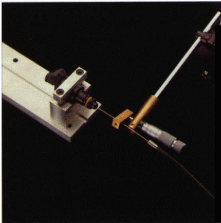
With frequency response from dc to 150 kHz, the Fotonic Sensor is ideal for analyzing squarewave and complex motions. The MTI-2000 is used here to measure the absolute travel and bounce of a fuel-injector valve.
