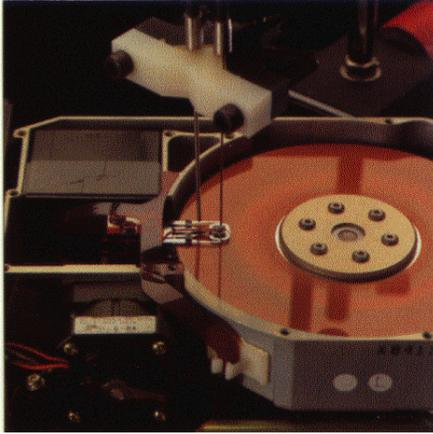
Two fiber-optic probes are used to perform modal analysis on a computer read/write head. With a high frequency response that makes it possible to measure both displacement and phase, the Fotonic Sensor has been chosen as the best instrument for this type of analysis by measurement experts in the U.S. and Japan.
