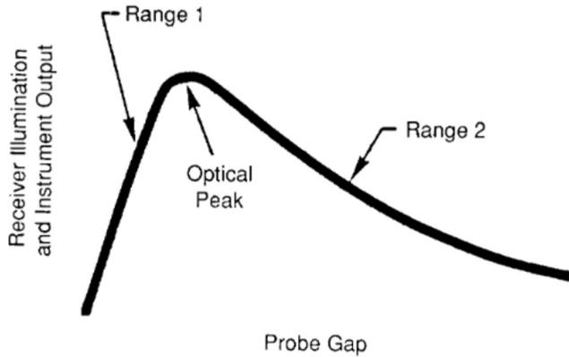
MTI-2000 Fotonic probe modules contain two sets of optical fibers. Light-transmitting fibers and light-receiving fibers are bundled together in three different configurations (random, hemispheric, and concentric transmit inside). Displacement measurement is based on the interaction between the field of illumination of the transmitting fibers and the field of view of the receiving fibers.
