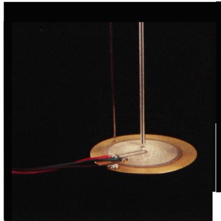
Two fiber-optic probes are used to measure surface displacement of a ceramic resonator. Fotonic probes are immune to electromagnetic interference (EMI) and operate effectively on a wide range of surfaces including nonmetallic materials, ceramic, glass, plastics, and composites.
