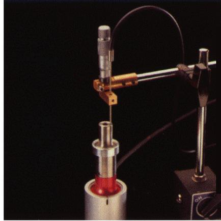
The Fotonic Sensor accurately measures the vibration amplitude of an ultrasonic welder tip at high frequencies and accelerations.
