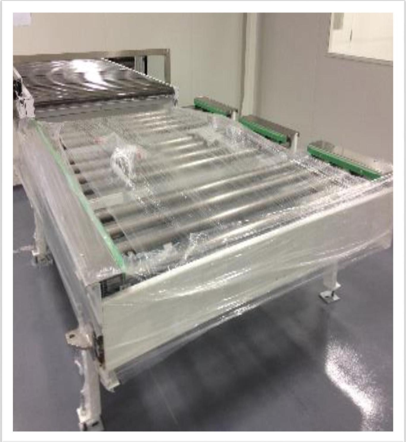
**Picture 4b: End Conveyor with position detectors and VFD.
