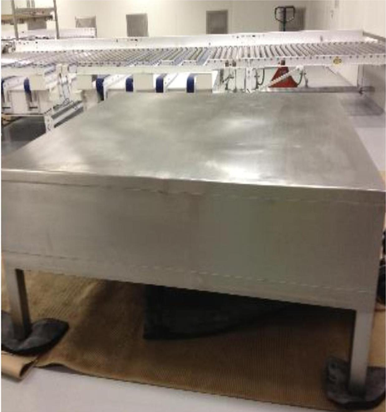
**Picture 4a: Cooling table. Table is cooled with Chiller water.
