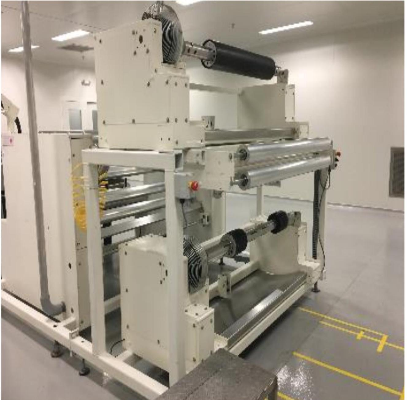
**Picture 2a: Unwinder for 2 rolls, breakers, roll diameter measurement & accumulator for roll change**
