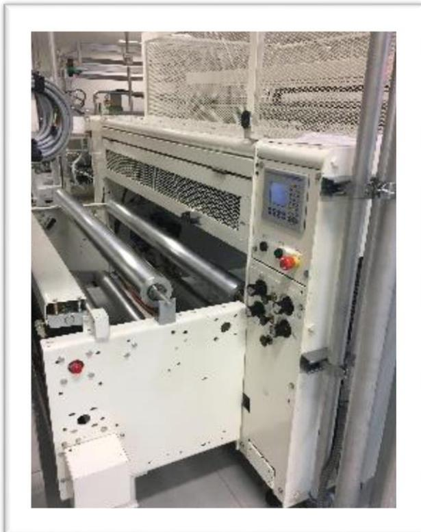
Picture 2d: Panel view for unwinder & cutting machine
