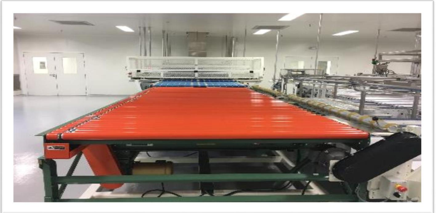
Picture 2c: Exit conveyors to send out blanks
